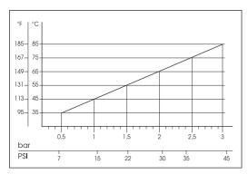
Naturally if the application allows to feed the pump with 3 bar (45 PSI) even at low temperatures (for example: 45°C - 115°F) the life of the wet end of the pump will be even longer.
