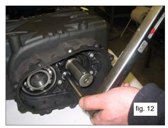
Insert the crown into the pump shaft, apply the washer and use the wrench (Fig.13) to tighten the screws to the torque level indicated in section 10.
