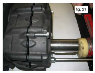
Using standard tools, remove the gear housing lid and take the bearing out of the pinion (Fig.22). Remove the crown screws and washer and extract out the crown. If necessary, use a percussion extractor on the two M8 holes (Fig. 23, position) or a standard extraction tool (Fig.23).
