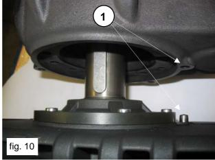
Fasten the gear housiong with the 6 M8x50 screws and tighten the latter with a torque wrench (Fig.11, and 12) as indicated in section 10 below.
